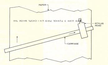
Fig. 1. The stylus head is mounted on a tilted carriage. As the paper advances, the stylus head moves up at the same rate, resulting in a level line of print. This eliminates the start/stop mechanism found in most printers.
